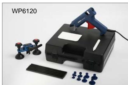
The repair method is simple : a Glue Tab is bonded to the centre of the dent with a special glue. With the help of the WPT Dent Puller the dent can be pulled out in a fluent, controlled way.
